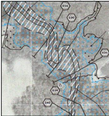
**Because of the high density of mass points, LIDAR is superior for automated Hydrologic and Hydraulic (H&H) analyses and automated floodplain delineation such as that shown to the left, which is used to create Flood Insurance Rate Maps (FIRMs).**
